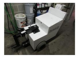
Rountine PM - Make sure the battery pack is not leaking. Check battery connections for corrosion, clean if needed. Check wheel bearings for dirt, properly greased. Check controls to make sure all connections and functions are working properly.
